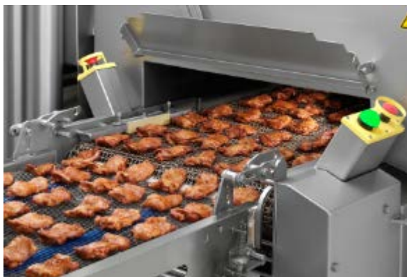
3. Smoked chicken thighs on the outfeed of the 3 rd Generation GEA CookStar
